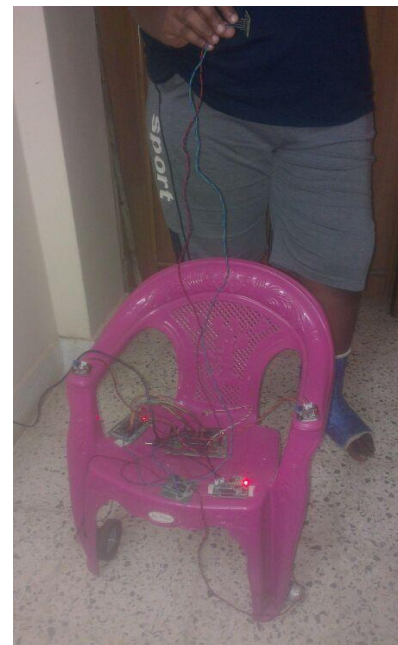
Fig 8: Steering of the wheelchair using the accelerometer
